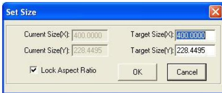
Input the target size on the X, Y axis, and click “OK” to change the size of the graph.
