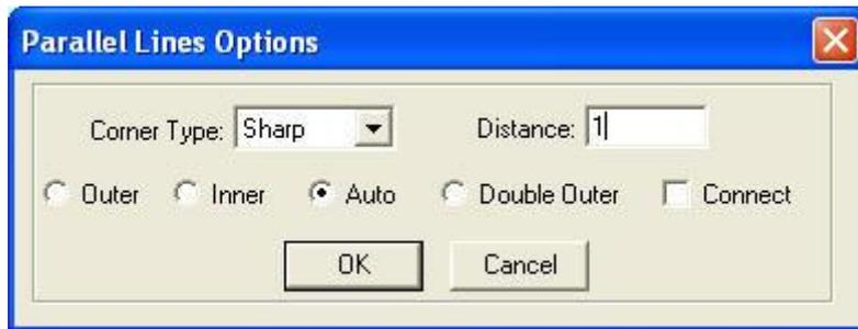
Select the needed option to generate parallel lines on a new layer. As it shows below:
