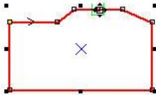
Move the mouse on the node and drag the mouse will change the shape of the graph.
