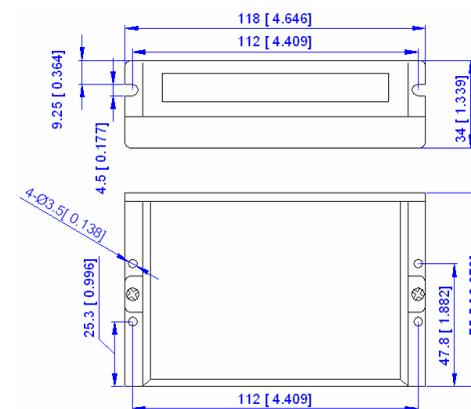
Figure 1: Mechanical specifications
