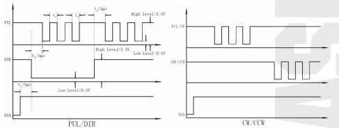
Figure 10: Sequence chart of control signals
