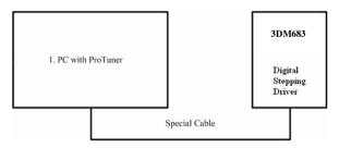
Figure 19: RS232 interface connection
