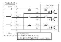
Figure 3: Connection to PNP signal (common-cathode)
