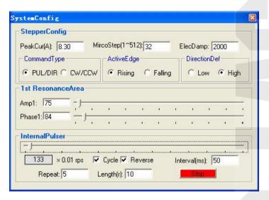
Figure 26: Anti-resonance tuning
