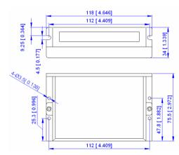
Figure 1: Mechanical specifications
