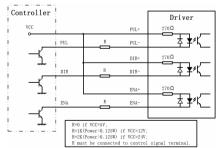
Figure 2: Connections to open-collector signal (common-anode)
