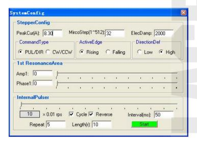
Figure 25: SystemConfig window
