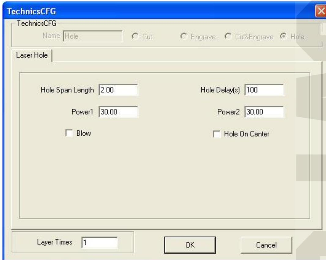
**Hole Span Length:** distance between two adjacent holes.
