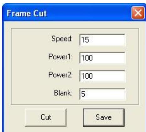
**Speed:** operating speed of the laser head in cutting. Different speed can be set according to the materials. It is better to define proper speed through testing.
