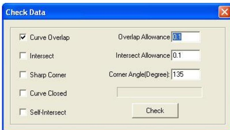
If abnormal phenomenon appears in the processing (such as fail to engrave, cut twice), use the tool to check all the data. Abnormal data checked will be shown as red. You can delete it or edit the node.
