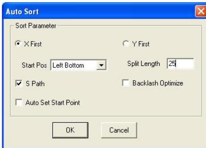
Divide height value 25 means the whole graph is divided into 6 sections (25mm\*25mm). The 6 area run along 1→2→3→4→5→6.
