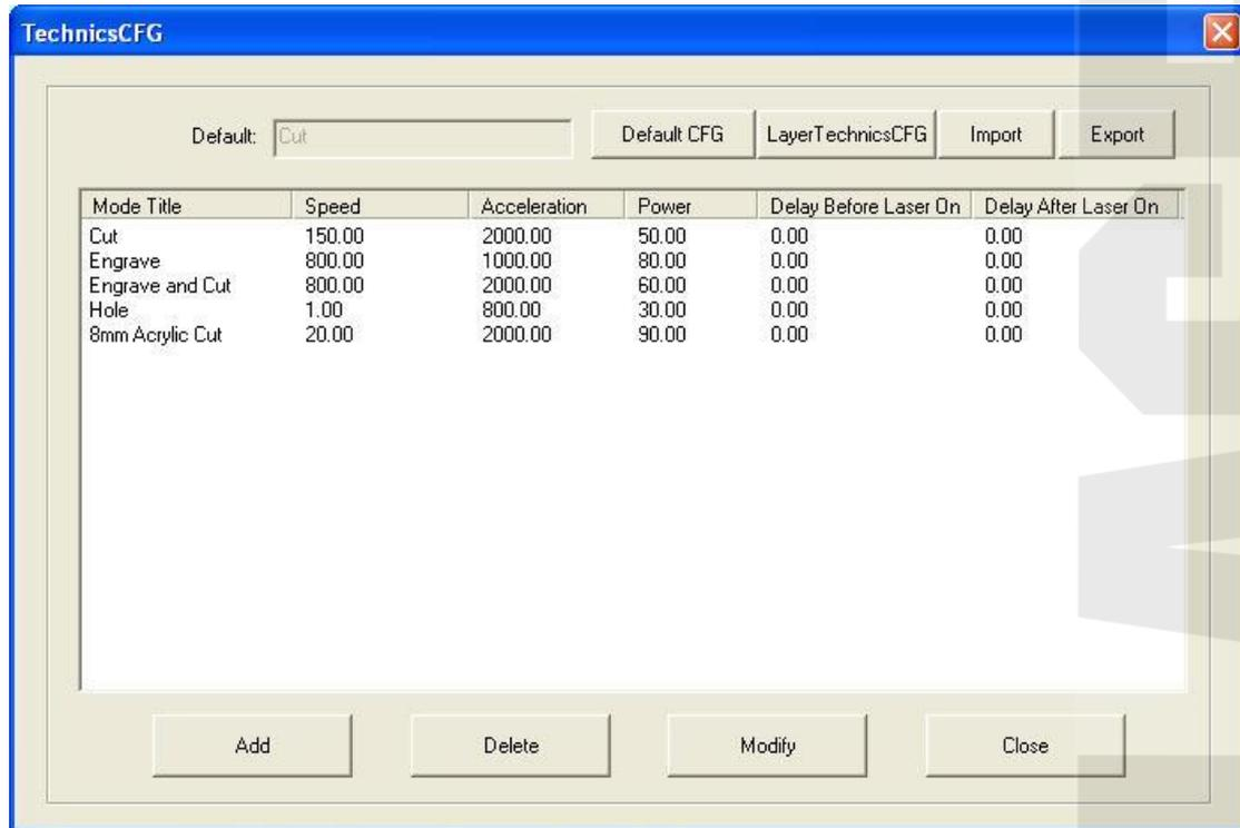
**Default CFG:** If “Cut” is set to be default CFG, system will set the process mode as “Cut” automatically when create a new file.
