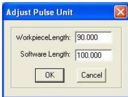
As the above picture indicate, draw a line in the software that the length is 100mm and cut. Measure the workpiece and the actual length of the line is 90mm, and input the value, the system will calculate the pulse unit automatically.
