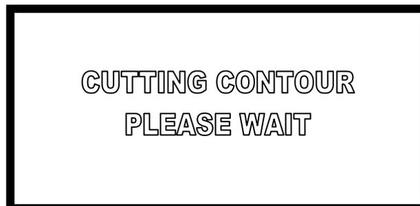
When the machine is cutting contour, only **START** and **STOP** can be used. It will return to the main interface once the motion completed.
