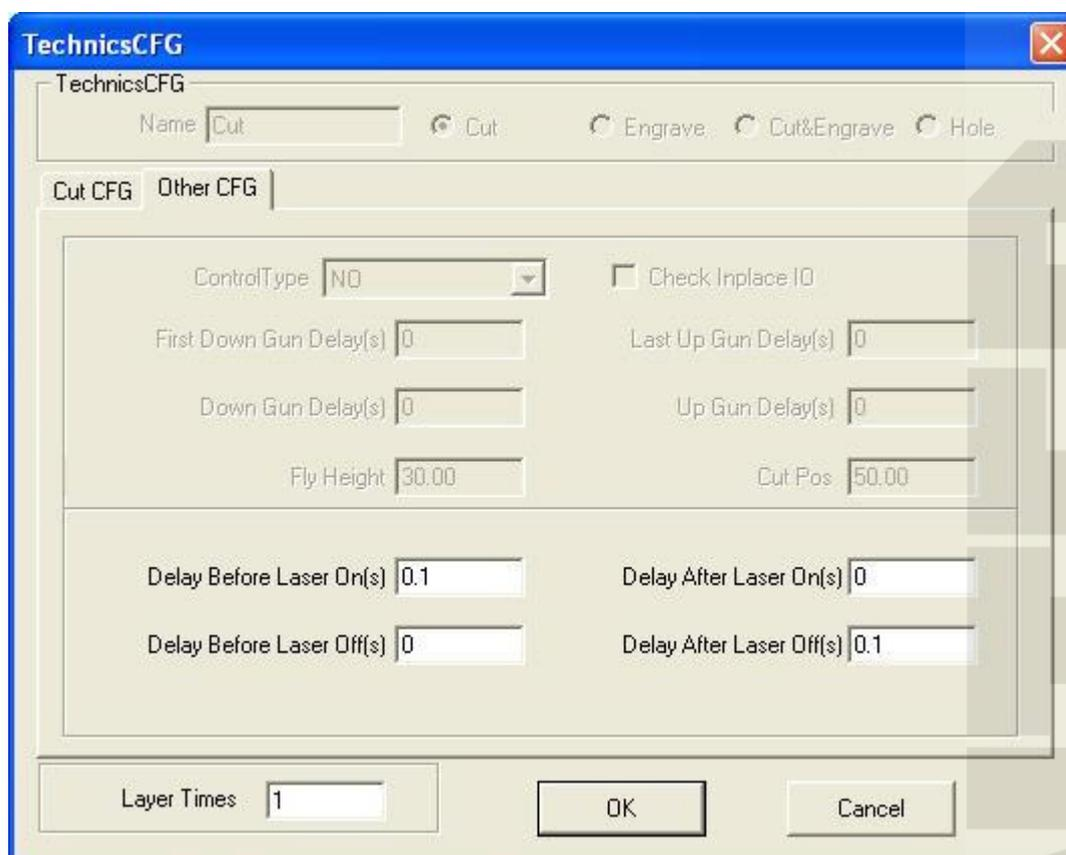
**Delay before laser on:** set the delay before the laser is on
