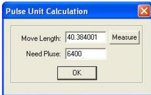
40.384001 in the picture above means the distance of the laser head moves every round of the motor is 40.384001 mm. 6400 is the pulse every round of the motor needs.
