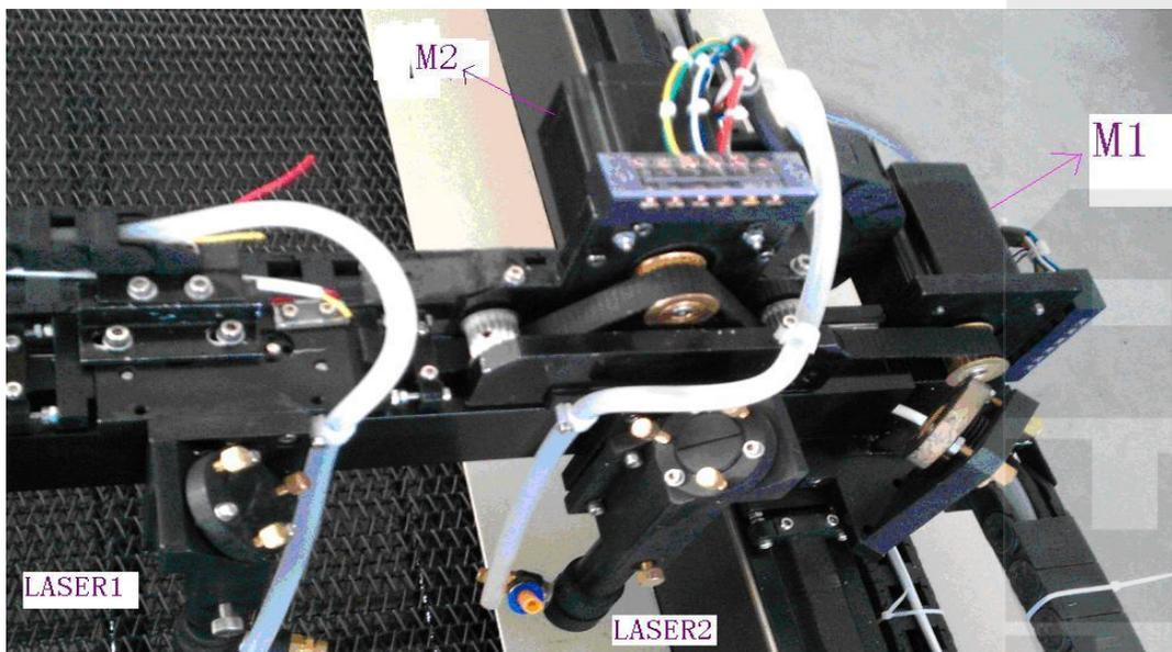
There are 2 laser heads on the X-Axis and they are fixed on one belt.
