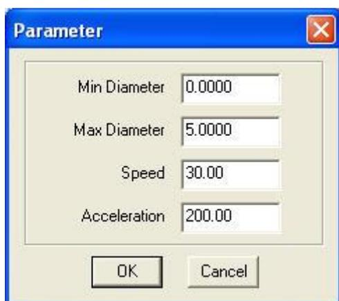
**Min diameter, Max diameter:** range of the circle’s diameter.
