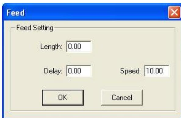
**Length:** after each processing, Z-Axis will feed a relevant distance for the feeding of the materials.
