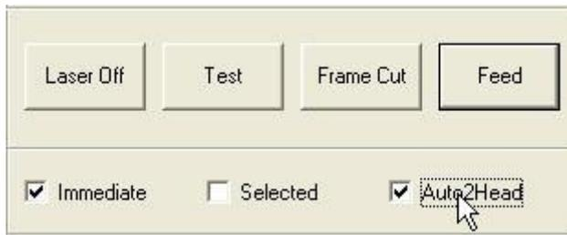
If the machine has automatic separation function, select this option and the space between the two laser head will adjust automatically; or the space between the two laser head won't adjust and the machine will be used as simple double laser head machine.
