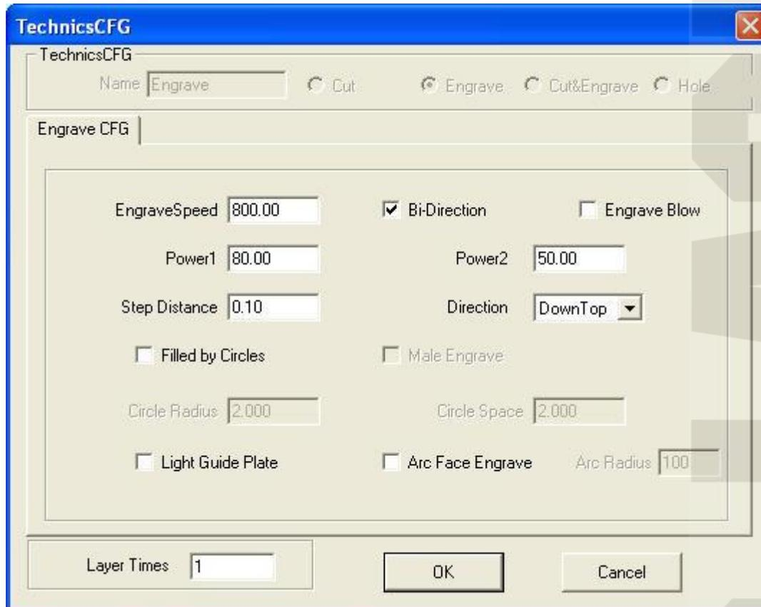
**Engrave Speed:** engraving speed on X-axis.
