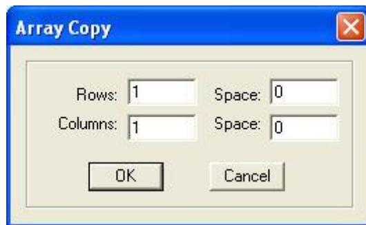
Input relevant parameters, identical graph with the number of the “lines × columns” will appear on the screen. The space between the graph will be determined by the “Space”.
