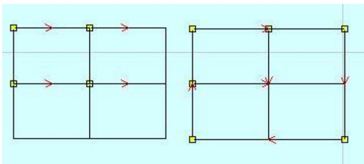
The left side is made up of 4 rectangles and the right side is processed. There are only 6 lines. This is very useful for array copy rectangles to improve the processing efficiency.
