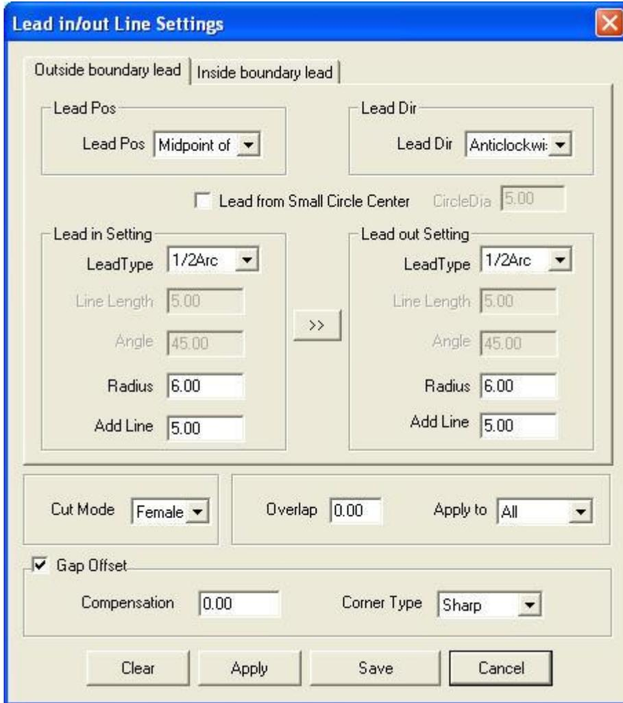
**Lead Pos:** set the situation of adding lead line.
