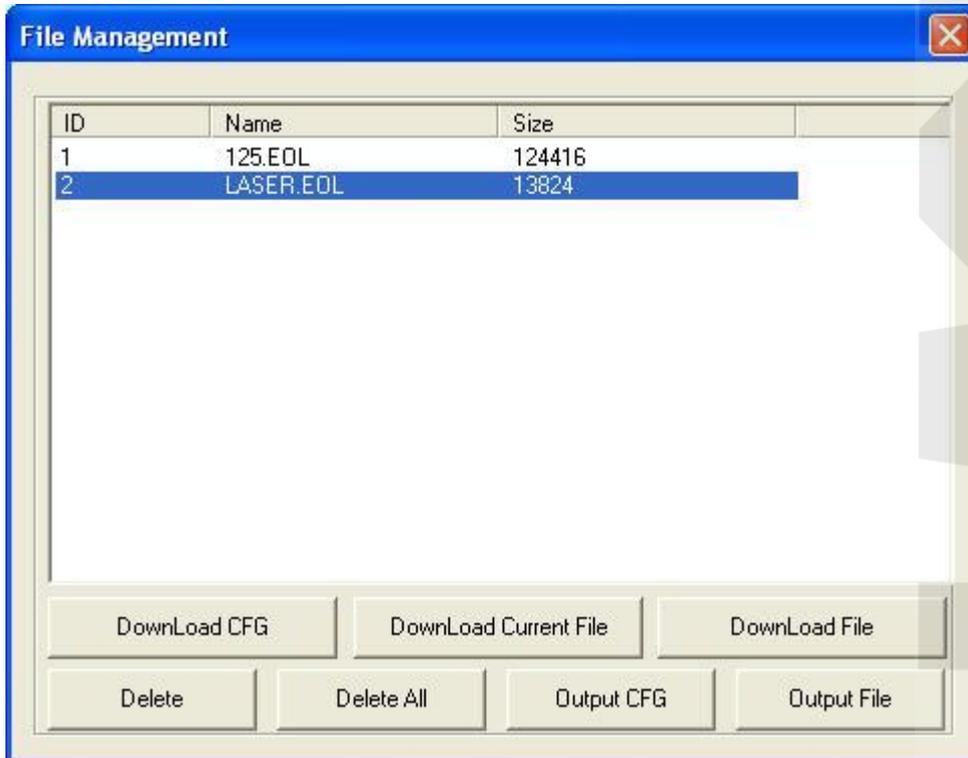
**Download CFG:** Download parameters of the machine to controller.
