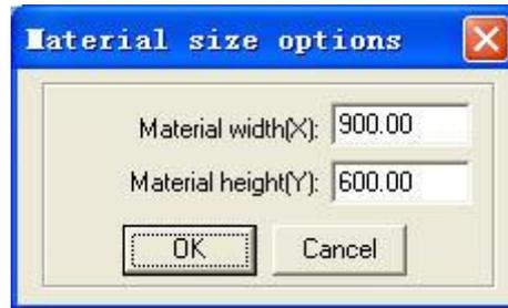
**Material Width:** width of the materials to process (default as the width of the worktable).
