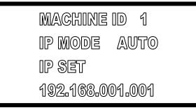
When the mode is "STATIC", you can input any number to identify different machine.
