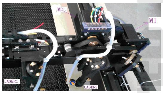
There are 2 laser heads on the X-Axis and they are fixed on one belt.
