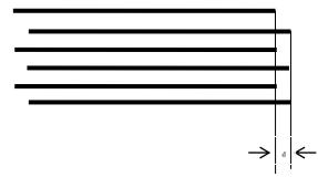
There is Backlash Compensation set in the Engrave Set of the Machine CFG. The backlash can be negative or positive value. Change the engrave step to 2mm, backlash 1mm, and start processing. If d increase, change it to a negative value; if d decreases, increase the number. Gradually d will near 0 after several adjustments. The value of the Backlash Compensation differs from different speed; you should set it according to different speed range.
